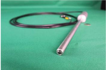
A Raman instrument interfaced with a fibercoupled probe, as shown here, given it the versatility and flexibility for measurements to be made in situ for the monitoring of processes. Unlike flat optics, where fouling is a challenge, the spherical interface minimizes sample buildup.
